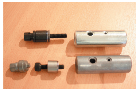
The internals of the mandrel have been modified for increased strength. The RNHT410 is shown at the top of the picture, with its predecessor underneath.
