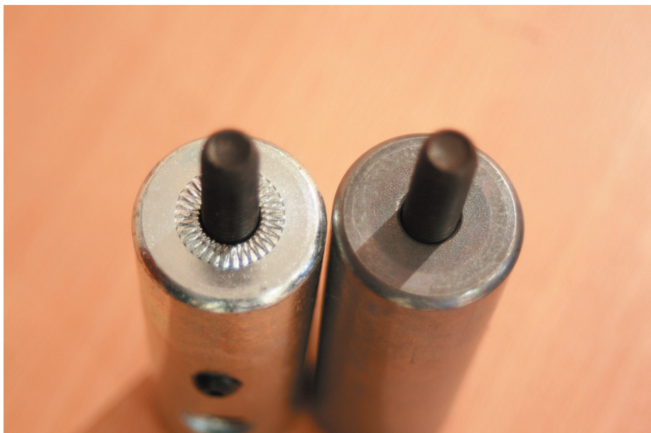
Here you can see the diamond-cut knurling on the RNHT410 (left) compared to its predecessor on the right.
