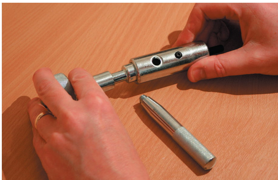
To assemble, slide main driver into mandrel of choice.
