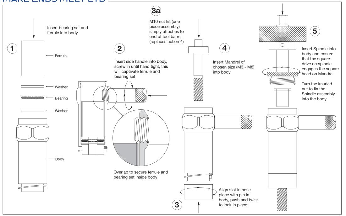
Note: Top 10mm Hex can be used to apply spanner/wrench to assist with larger sizes Push Spindle into body and ensure that the square drive on spindle engages  $\bigcirc$ the square head on Mandrel 6
